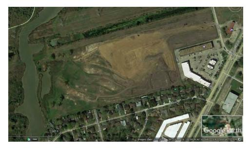
When we compare the January 2019 photo below with previous photography, we see discoloration from a sediment plume migrating off the construction area into the lake and wetland adjacent to the construction site, and further polluting Robinson Bayou. By filling and regrading much of the area containing wetlands documented in the National Wetlands Inventory, Broad Reach caused muddy water to flow over the site and into the jurisdictional wetlands that remained intact, as well as Robinson Bayou.
